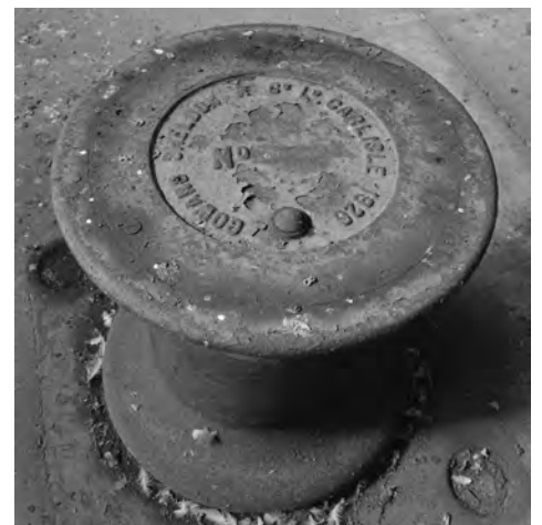
Fig. 71. BB96/03865. Devonport South Yard South Smithery (S126) photograph of Cowans Sheldon driven capstan (1926) (29 Feb 1996). ©Crown copyright.HE.
